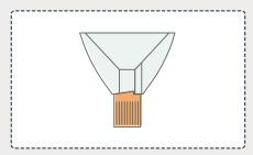
5 Make sure the funnel is in the correct position: the notch on the orange adaptor has to be against the stop notch of the funnel.
