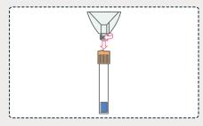
4 Screw completely the funnel onto the adapter.
