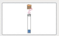
3 Screw the orange adapter onto the sample tube, making sure that the notch on the adapter is pointing up.
